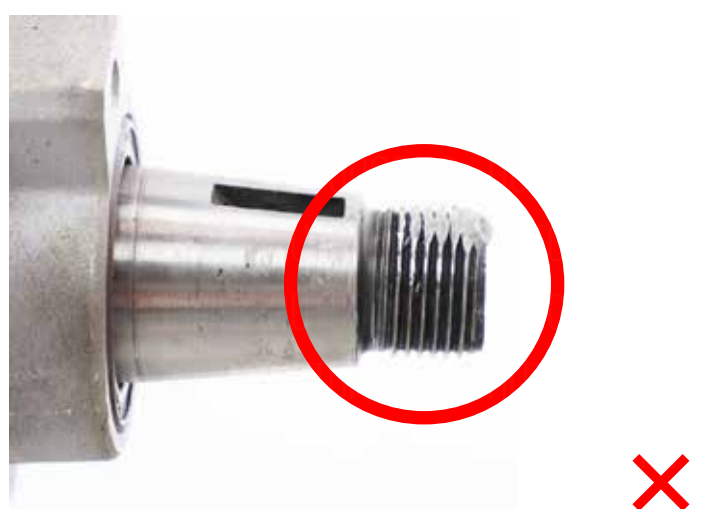
Damaged drive shaft
