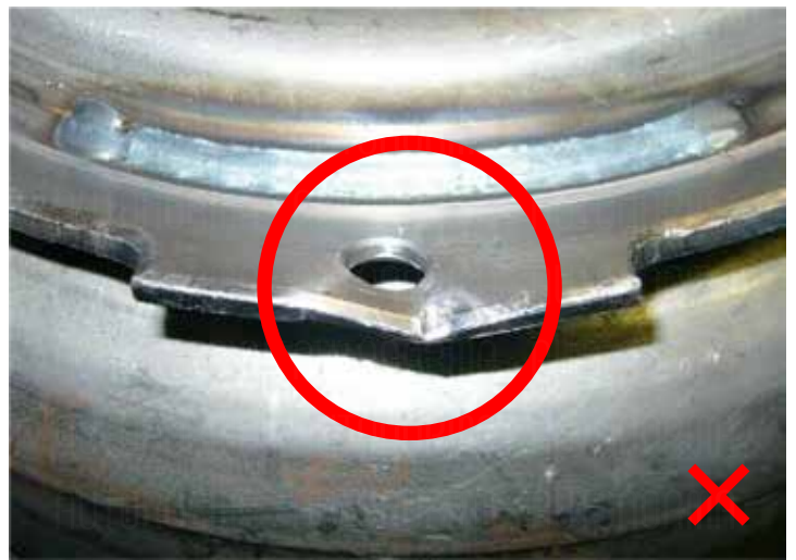
Damaged mounting rim
