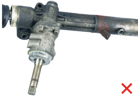
Broken or missing pipes
