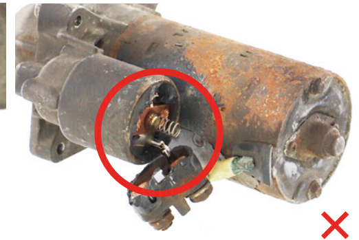
Damaged connector – broken
