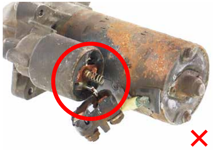
Damaged connector – broken
