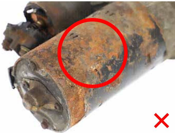
Missing / illegible labeling
