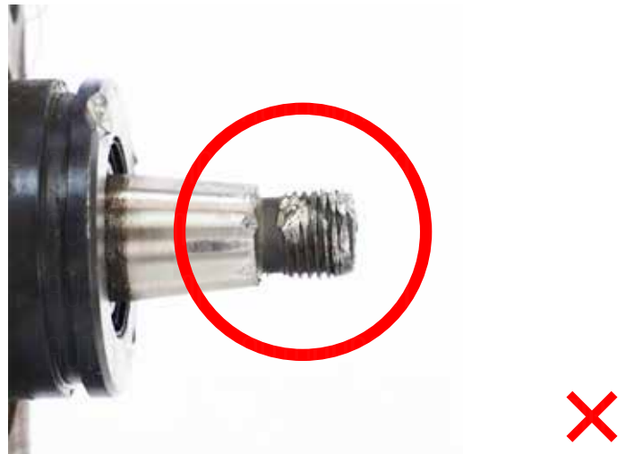
Damaged drive shaft
