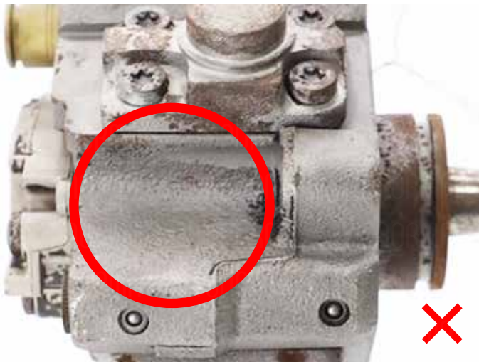
Corrosion at the drive shaft
