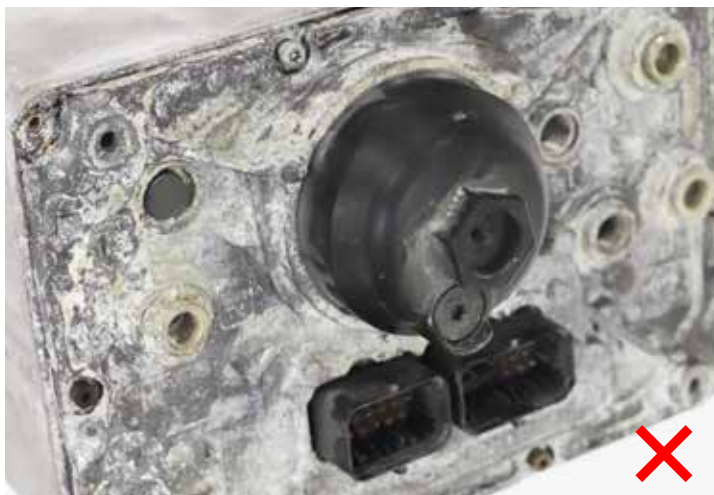
Part damaged by AdBlue urea
