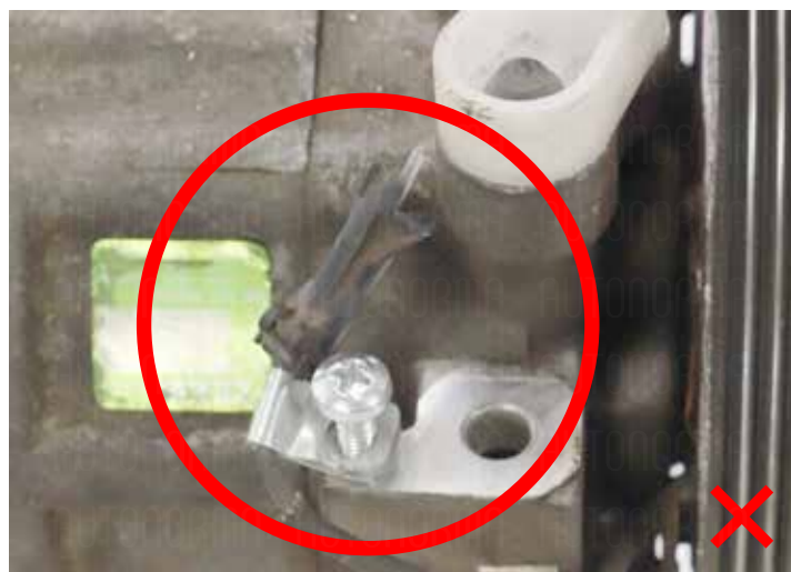
Damaged / missing connector
